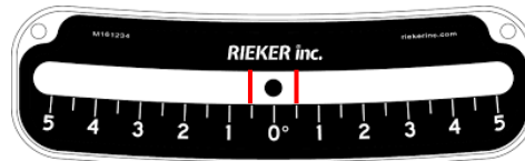
Figure C-12 - Inclinometer during Operation
